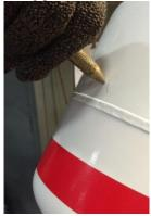
Figure 4. Placement of Non-sparking Pick for Piercing
