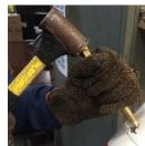
**5.4.1.2** With a hammer or mallet, lightly tap the handle of the non-sparking pick to pierce a hole in the side of the tank (see Figure 5).
