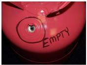
Figure 3. Open Rupture Disc
